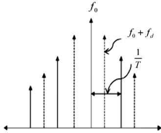
Fig. 18. Waveform used by the pulse radar system in frequency domain.
