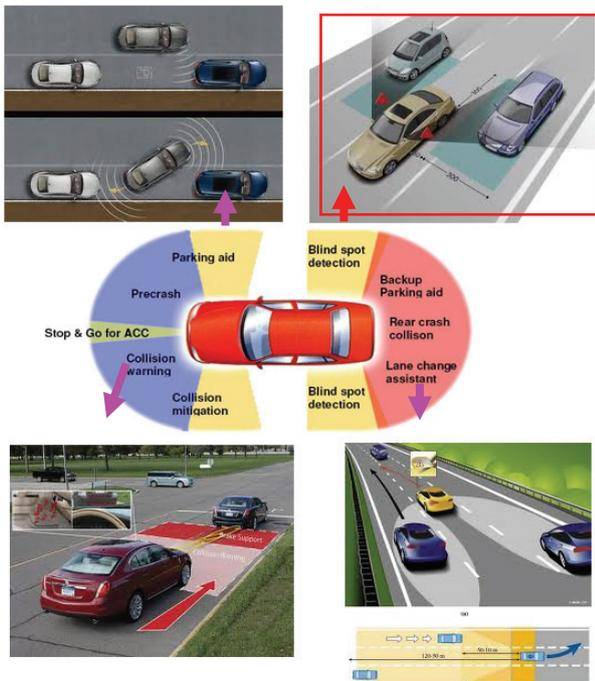
Fig. 9. Applications using short-range radar sensor.
