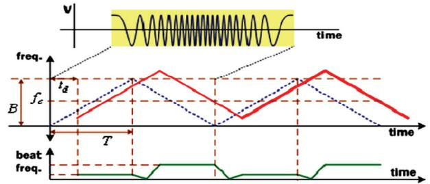
Fig. 15. Triangular wave of FMCW radar.
