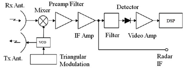
Fig. 14. Structure of FMCW radar system.
