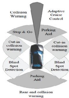
Fig. 4. Safety system using radar sensors around a vehicle.
