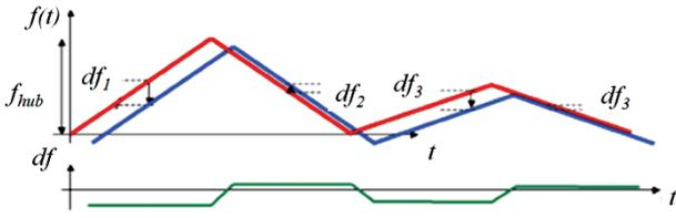
Fig. 26. FMCW radar waveform (red) and the corresponding target return signal (blue) for a single target.
