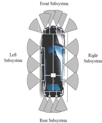
Fig. 3. Radar sensors around a vehicle.
