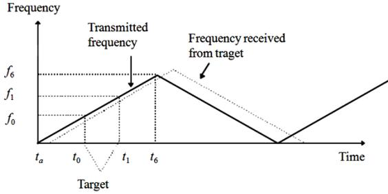
Fig. 29. Triangular waveform FMCW radar system.
