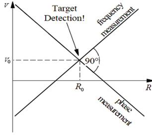
Fig. 34. Graphical resolution principle of ambiguous frequency and phase measurements.
