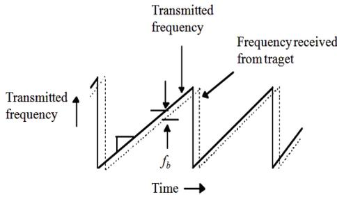
Fig. 28. FMCW saw-tooth waveform.
