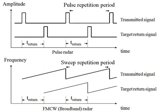
Fig. 40. Radar waveforms.
