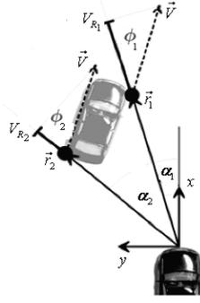
Fig. 37. Graphical representation of TV ranges and angles.
