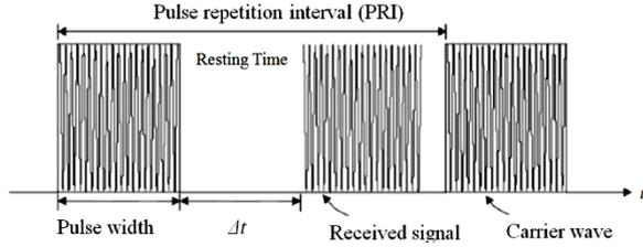
Fig. 17. Waveform used by the pulse radar system in time domain.
