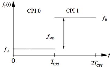
Fig. 32. FSK modulation principle.
