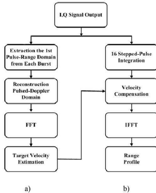
Fig. 22. Stepped-frequency pulsed-Doppler signal processing algorithm block diagram: a – signal processing algorithm to define the relative velocity; b – signal processing algorithm to define the range.
