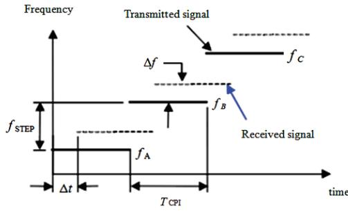
Fig. 23. FSK signal waveform.
