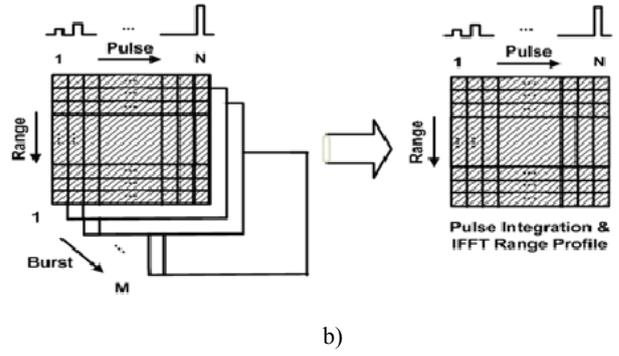
Fig. 21. Stepped-frequency pulsed-Doppler signal processing algorithm: a – signal processing algorithm to define the TV velocity; b – signal processing algorithm to define the range of target vehicle.
