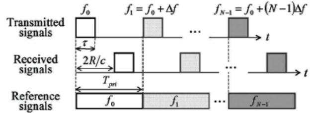
Fig. 20. SFPD radar system signal waveform
