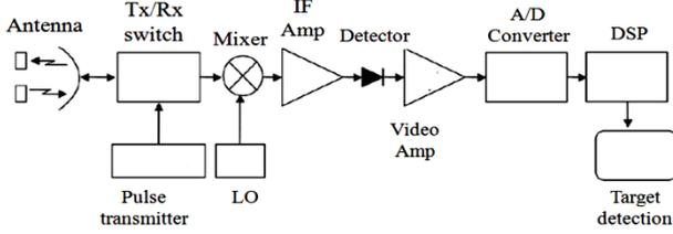
Fig. 16. General structure of pulse Doppler radar system.
