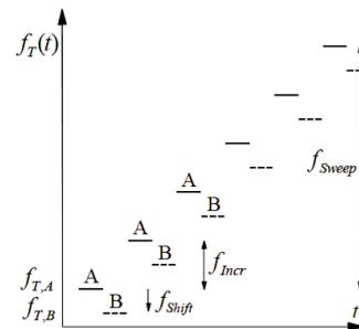
Fig. 33. Combined FSK-LFMCW waveform principles.
