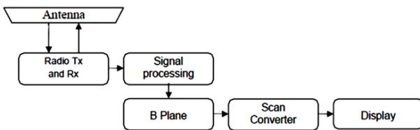
Fig. 39. Block diagram of typical radar sensor system.
