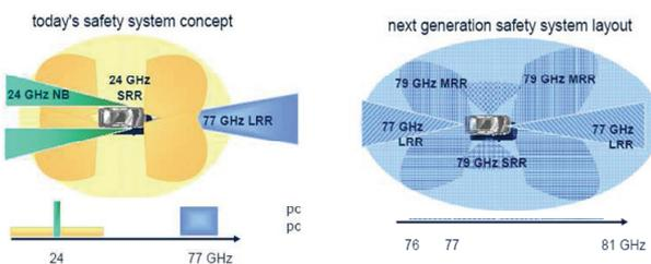
Fig. 10. Synergies within higher frequency bands.
