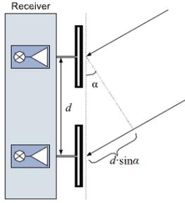
Fig. 31. Antenna array in receive mode.
