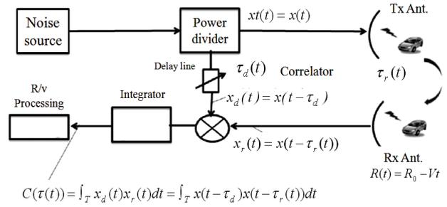
Fig. 24. Simple flowchart of random noise radar system.
