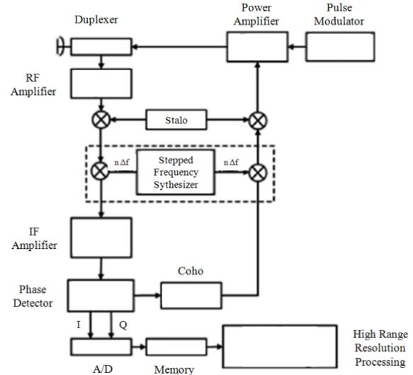
Fig. 19. Structure of SFPD radar system.
