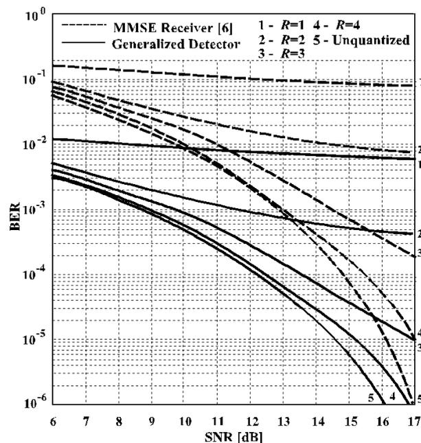
Fig. 2. BER for the uniformly quantized and sampled CDMA signal with multiuser generalized detector and perfect control.  $N = 64, K = 32$ .
