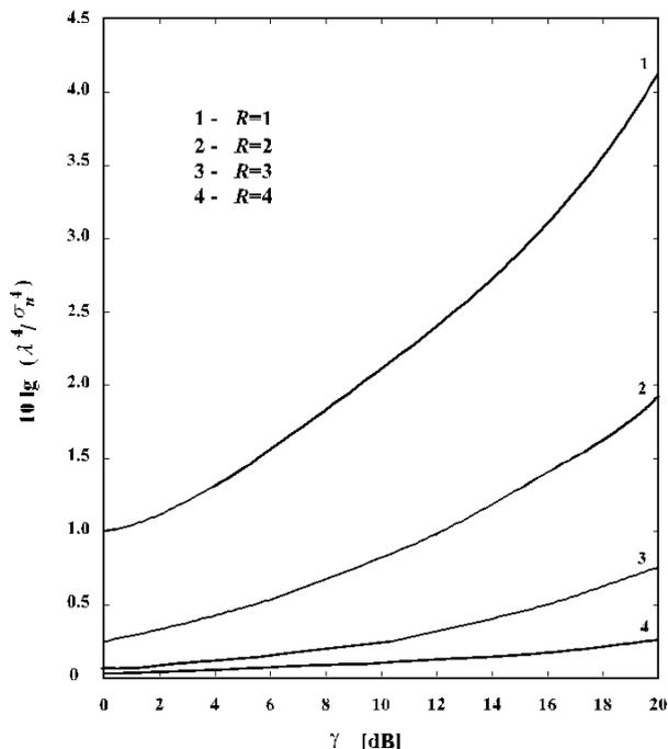
Fig. 1. The normalized equivalent noise variance  $\frac{\lambda^4}{\sigma_n^4}$  versus the sum of SNRs.
